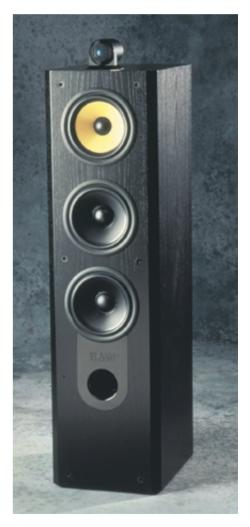
Description 2 way vented-box system **Power Handling** 50W - 250W into 8 ohms on **Drive Units** 1 x 25mm metal dome  $\cdot$  high frequency unclipped programme 1 x 165mm Kevlar\* - midrange Height: 1017mm Width: 258mm Dimensions Depth: 334mm 2 x 165mm Cobex® - bass Frequency Response 35Hz - 20kHz ± 3dB on reference axis Finish Black Ash, Walnut, Rosewood Sensitivity 90dB spl(2.83V 1m) Grille: Black Cloth Nominal Impedance 8 ohms (minimum 3.7 ohms)
