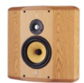
Description 50W - 120W into 8 ohm on unclipped 2-way closed-box system Power handling Drive units 1 x 25mm alloy dome high-frequency programme 1 x 165mm woven Kevlar® cone Dimensions Height: 394mm Width: 392mm bass/midrange Frequency response 75Hz – 20kHz ± 3dB on reference Finishes Cabinet: Real wood veneers, Black Ash, Cherrywood, Red Stained Cherrywood axis Sensitivity 90dB spl (2.83V, 1m) Grilles: Black cloth
