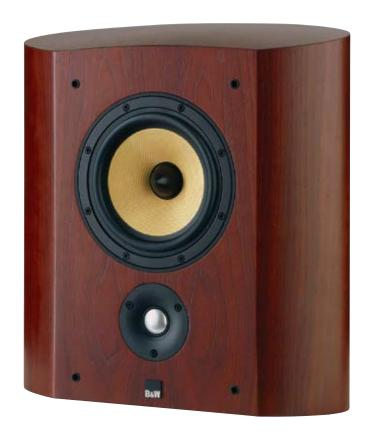
The SCMS features essentially the same driver complement as the 805S. It's a 2-way system with a Kevlar® cone bass / midrange driver and aluminium dome tweeter. Here, though, the cabinet is much shallower so that it can be mounted on-wall with the minimum of intrusion into the living space. The system is also balanced for its intended on-wall application, taking into account the bass reinforcement from the rear wall.
