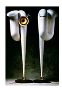
Description Fourth-order vented box 50W - 120W into 8 ohms on unclipped Power handling **Drive units** 1 x 25mm (1-inch) magnetic fluidcooled, metal dome - high frequency Dimensions Height: 1370mm 1 x 165mm (6.5-inch) high powered Width: 420mm Keylar® cone - bass/midrange Depth: 360mm Frequency response 49Hz · 20kHz ± 3dB on reference axis Finishes Gloss White, Gloss Black 87dB spl (2.83V 1m) Sensitivity Nominal impedance 8 ohms (minimum 4 ohms)
