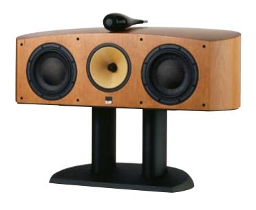
The HTM3S is the larger of the two centre speakers that feature our improved aluminium dome tweeter. The HTM3S also features two 6.5" Rohacell® cone bass drivers in a symmetrical arrangement with a central Kevlar® cone FST™ midrange driver.
