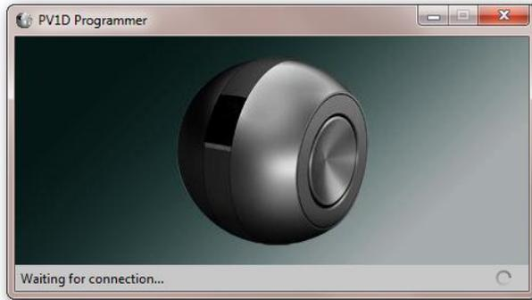
4. Connect the PV1D to mains power. It will assume a state ready to receive a firmware update. The navigation buttons will illuminate, but the display screen and LED will remain dark. At this point, your computer may install driver software, after which the Programmer will continue and install the new firmware. When the installation is complete, its window will look like this:
